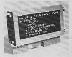
This enables the depth of the display to be dramatically reduced to less than one inch, giving new scope to the
