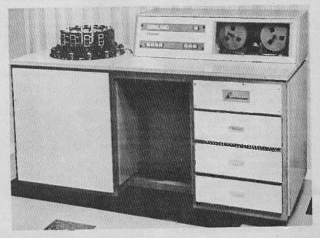
Fig. 9. "Discomatic" produces cropped discs from paper tape control.
