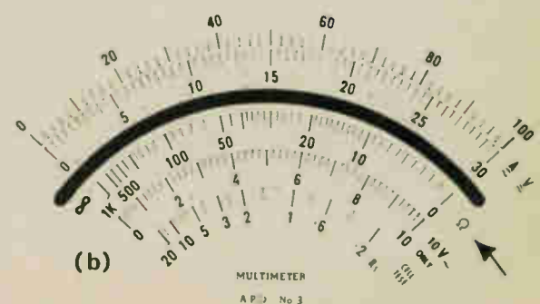
Fig. 5(a). The circuit required to measure ohms. (b). A typical multimeter scale - The Ohms scale is the centre one.
