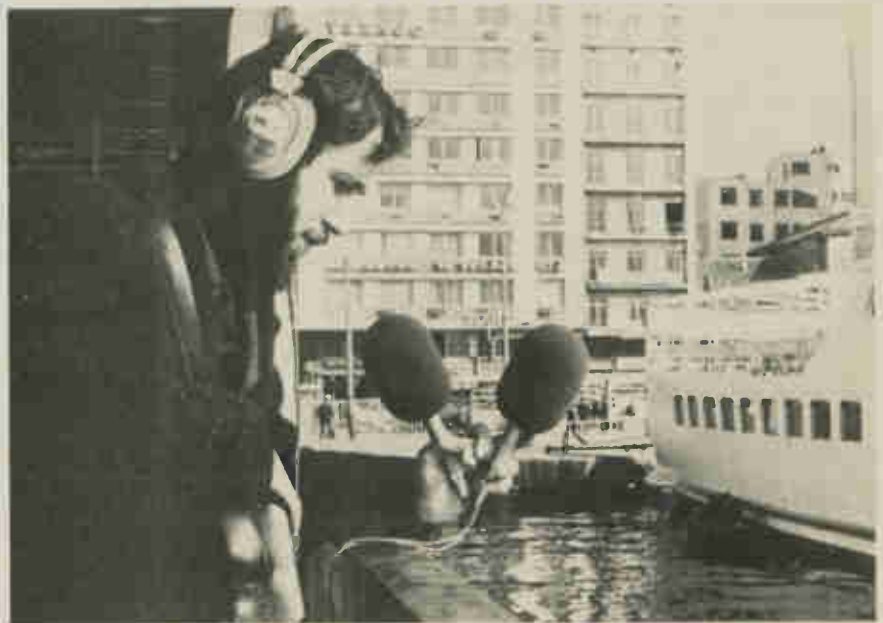
Recording the departure of a ship from Piraeus Harbour (Greece). Equipment used to make this stereo recording includes Neumann KM76 condenser microphones and windshields. Sennheiser headphones are being used to monitor the output from the Stellavox SP7 recorder.
