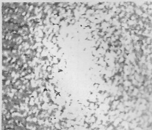
Complex pattern of dots produced by passing laser beam through frosted glass.
