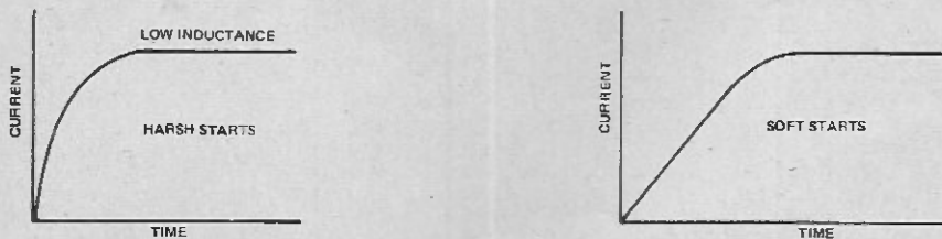
Fig. 2. The amount of in-line inductance alters the harshness of the weld attack.
