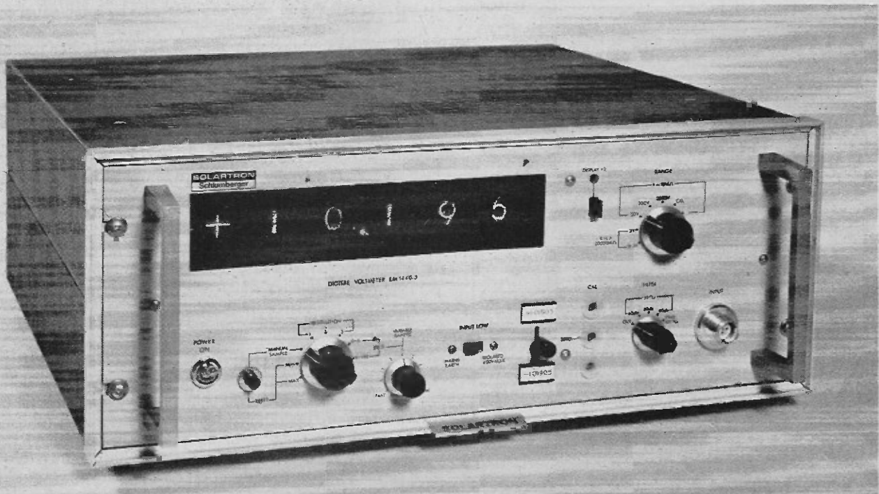
This digital voltmeter from Solartron has variable sampling speeds.
