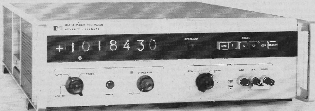
Hewlett-Packard's 3462A digital voltmeter uses potentiometric-integrating principle.
