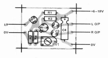
Above is the component overlay of the complete device, below left is the PCB pattern shown full size  $(45 \times 34 \text{mm})$ . Neat layout of the prototypes can be seen clearly in the photograph below.
