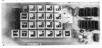
The assembled Scrumpi 3 kit. The system's firmware is resident in the two EPROMs seen top left with their protective labels. The three presets we had to fit to get the video levels right can be seen bottom centre.
