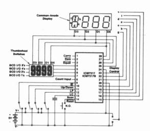
Fig. 1. The 7217 (common anode) version. The display and power connections are the same for the 7217B, 7227 and 7227B.
