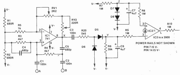
Fig. 1. Main circuit diagram of the proximity switch.
