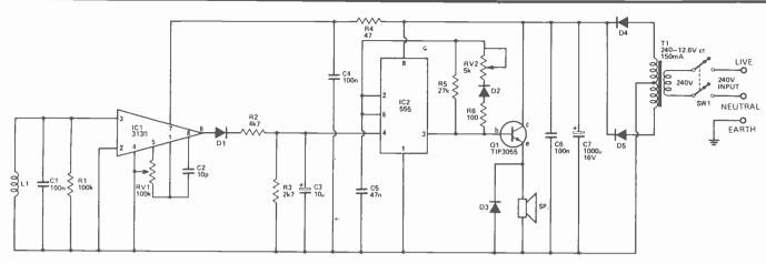
Fig. 1. Full circuit diagram of the tele bell extender.
