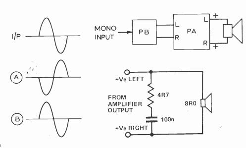
Fig 1. On the left is a diagram showing the input and output waveforms from the Power bulge, as can be seen the two outputs (A and B) are 180° out of phase with each other. Above right is how to connect the unit to any stereo amplifier, the lower circuit shows additional components suggested to stabilise the speaker load.
