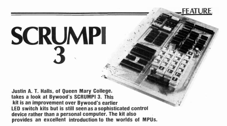
Srumpi 3 is the cheapest currently available microprocessor kit with full alphanumeric input and a VDU type display. It is the successor to the Scrumpi 1 and 2, switch and LED kits and is based on the same MPU, National Semiconductor's SC/MP. The kit also provides facilities for cassette and teletype interfaces.
