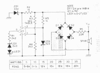
ferent input powers across an 8 ohm load. If different load values are to be used for the speaker the value of R3 can be determined from the equation,
