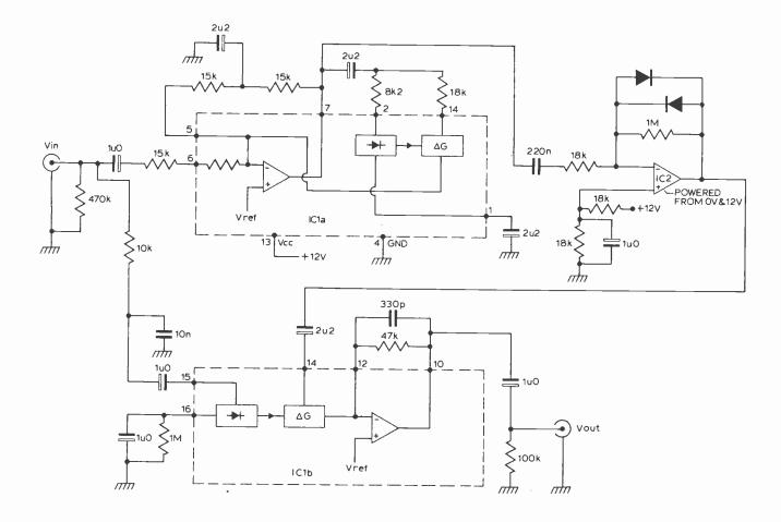
Fuzz boxes are used by guitarists to produce harmonic distortion and sustain. If you want to produce only the distortion, but to retain the original envelope of the signal then this is the circuit
