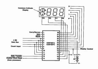
Fig. 2. The 7227A (common cathode) version. The display and power connections are the same for the 7227C, 7217A and 7217C.
