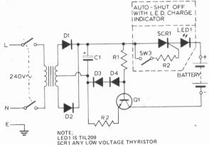
NOTE; LED1 IS TIL209 SCR1 ANY LOW VOLTAGE THYRISTOR R2 SELECTED TO GIVE ONLY ONE CHARGE RATE OF 45mA INSTEAD OF SIX POSITION RANGE SWITCH GIVEN IN ORIGINAL DESIGN
