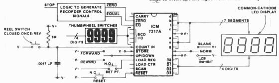
TAPE RECORDER POSITION INDICATOR/CONTROLLER This circuit shows an application which uses the up down counting feature of the ICM7217 to keep track of tape position on a tape recorder. This circuit is representative of the many applications of up/down counting in monitoring dimensional position.
