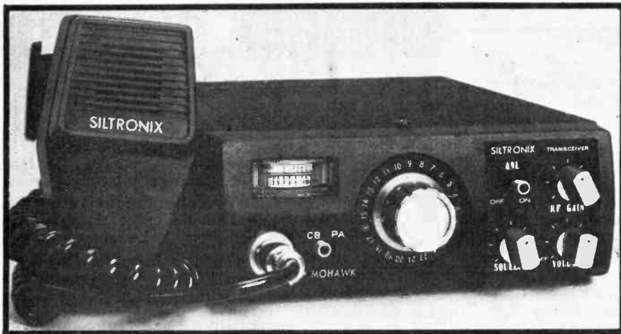
A full 23 channel CB rig of the type which is now in 25% of US cars. This is a deluxe type with noise limiter and RF gain control. This will put out the maximum signal of SW. Price is $ 169.95 (£93).
