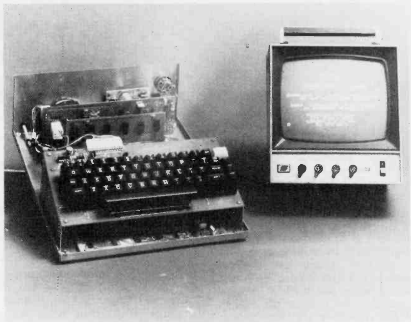
Fig. 2. The MEK kit uses a PIA and programmable timer as a teletype interface.
