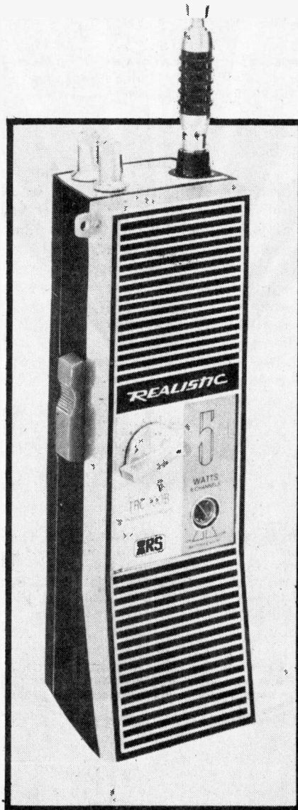
Typical of the more powerful hand-held units is this one from Radio Shack (North America's Tandy). This is supplied with a crystal for Channel 11 — five other channels can be switched in but crystals are extra. Cost is $89.95 (about £50).
