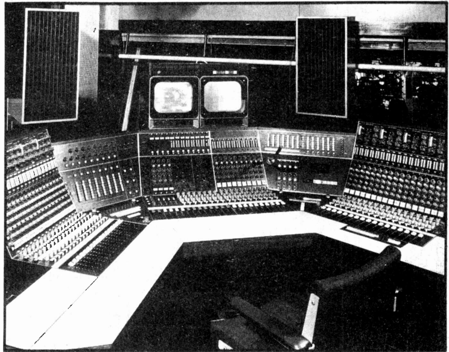
Fig. 2. A 44 channel broadcast console. Note the studio monitors in the background. The faders are in three groups along the front of each bank.
