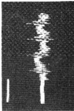
Fig. 4 (a). Above: the waveform of the Click Eliminator blanking pulse straddling the click (see Fig. 8). Below: the combined waveform showing the blank period inserted into the music.
