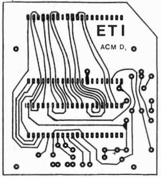
The Autoranging Capacitance Meter display board.
