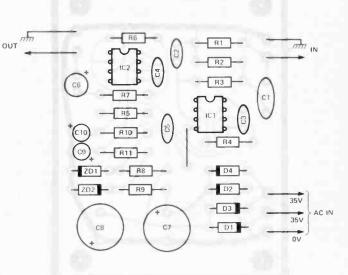
Fig. 1 Component overlay for the bridging adaptor.
