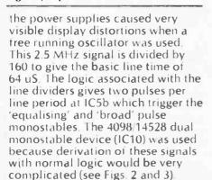
The line sync pulse is generated by the logic (IC4a) and a choice between this and the other two pulses is effected in ICs 5c and 9.
