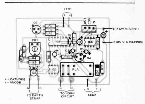
Fig. 3 Component overlay for the Car Alarm. There are a lot of polarised capacitors so make sure you get them all the right way round.
