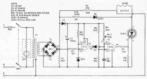
Fig. 1 Circuit diagram of the ETI Hotwire.
