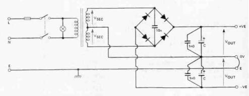
Fig. 5 Power supply for split rail amplifiers.
