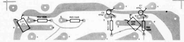
Fig. 3. This overlay shows the components which are mounted directly on the copper side of the PCB.
