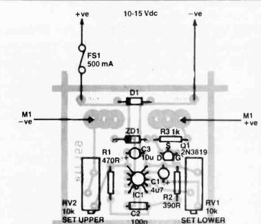
Fig. 2 Component overlay for the Voltage monitor. Note that IC1 is in a 10-pin T099 case.
