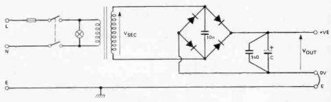
Fig. 4 Power supply for single rail and bridge amplifiers.
