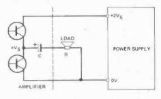
Fig. 2 Single rail configuration.
