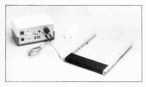
This easy-to-construct project is a controller for a hot-wire polystyrene cutter. This method of cutting foam polystyrene is probably better than most others as it does not create any rough edges or crumbs; it actually works by melting the material as it comes into contact with the hot wire.
