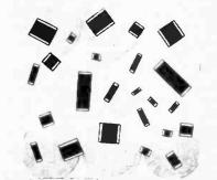
Fig. 3 Ceramic chip capacitors shown about actual size.
