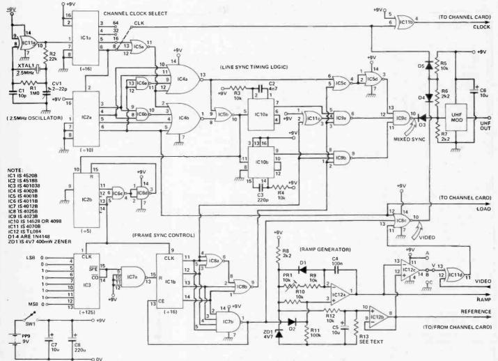
Fig. 9 Circuit diagram for the main board of the TV Bargraph.
