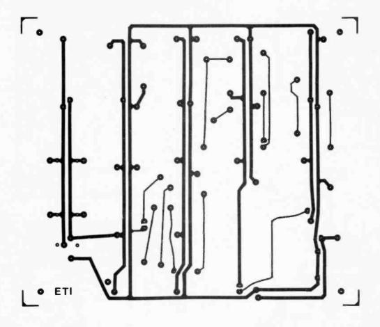
Above: the foil pattern for the top side of the Autoranging Capacitance Meter main board, which is double-sided. Below: the foil for the bottom side of the board.
