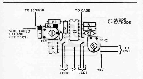
Fig. 3 Component overlay of the ETI Bodywork Checker.
