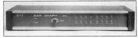
generate a display on a television screen consisting of a number of vertical columns. The height of each column is proportional to a specific input voltage. The columns may be upwards (positive) or downwards (negative) from a reference level. This reference may be changed if only positive-going signals are to be processed.
