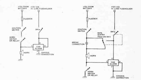
Fig. 2 Common horn circuits and how to connect the alarm to them. The circuit on the left will have only one wire from the horn. The one on the right is found in cars such as the Leyland Mini LS and is rather more complex.
