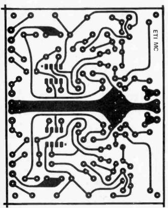
The moving coil PCB of Phono Amplifier.
