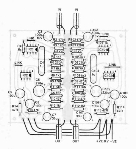
Fig. 3. Component overlay for the moving magnet stage.
