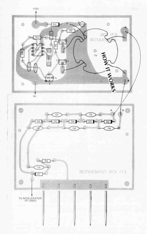
Fig. 2 Component overlay and wiring for the ion generator. The two-board design will allow for different physical layouts and connection pads are provided for experimentation with accelerators and off-board emitters.
