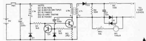
Fig. 1 Circuit diagram of the DVMeg insulation tester.
