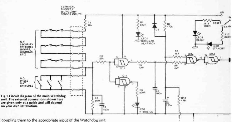
Anti-thug or panic protection systems enable the owner to activate the alarm system manually if he is attacked by thugs inside the house or suspects the presence of intruders in the house. Protection can be obtained by mounting normally-open push-button switches in readily accessible points near the front and rear doors and in the lounge and bedrooms and then wiring
