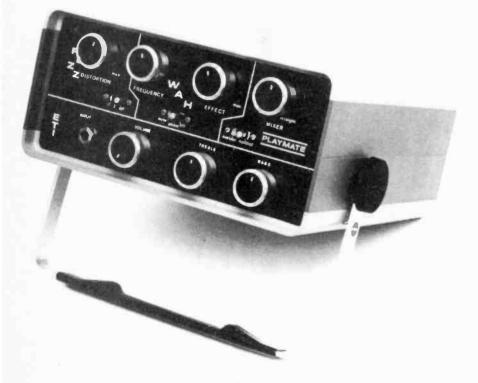
wah. After the effects stages, the dynamic range of the signal is restored to normal before being fed to the mixer, tone controls and power output stages.
