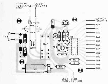
Fig. 1 Component overlay of the ETI Enlarger Timer.
