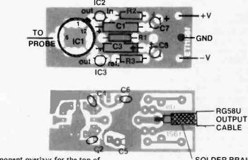
Fig. 2 Component overlays for the top of the board (top) and the bottom of the board (bottom!).
