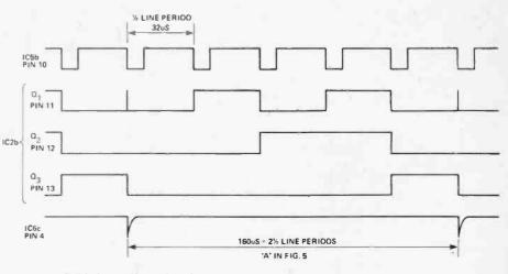
Fig. 4 The divide-by-5 effect of IC2b.
