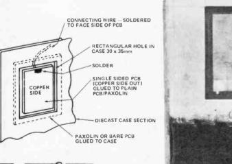
Fig. 1 This cutaway diagram shows the constructional details for the sensor plate.
