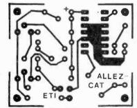
Pest Controller foil, ELECTRONICS DIGEST, WINTER 1983
