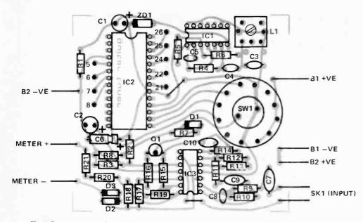
Fig. 2 Component overlay for the main PCB.
