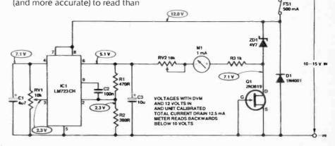
Fig. 1 Circuit diagram for the Voltage Monitor.
