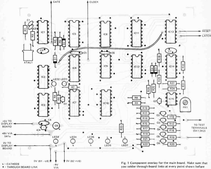
you solder through-board links at every point shown before mounting any components.
