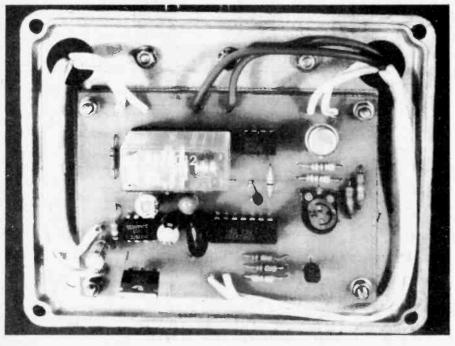
(Left) The completed unit was mounted on the lid of a diecast box with a scrap of blank PCB substrate underneath as an insulating spacer. The external leads are passed through two grommetted holes to a terminal block on the outside.
