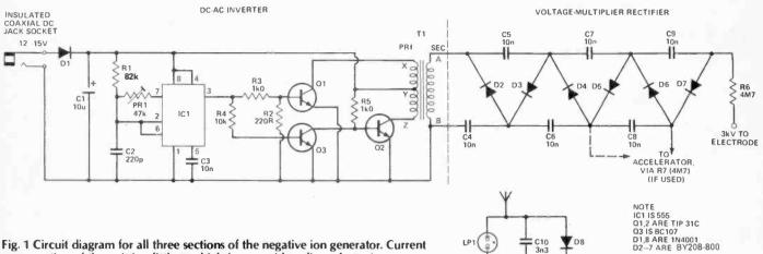
Fig. 1 Circuit diagram for all three sections of the negative ion generator. Current consumption of the unit is a little too high for use with ordinary batteries; we recommend you run it from a battery eliminator pack or a 12 V car battery.
