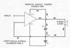
Fig. 2 Single-ended power amp showing how current flows in the power supply and the load.
