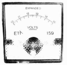
This simple, low-cost instrument can be built into power supplies or used as a portable or fixed 'battery condition' monitoring meter. Design by Simon Campbell and Roger Harrison.
