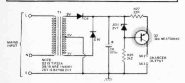
Fig.2 (Above) Circuit diagram of the trickle-charger.
