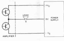
Fig. 1 Split rail power supply configuration.
