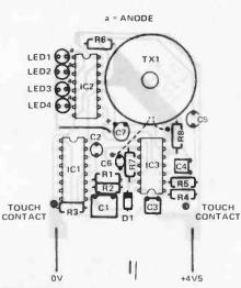
Fig. 1 Component overlay for the ETI Parking Meter Timer. You can't use sockets, so take care when soldering the ICs.
