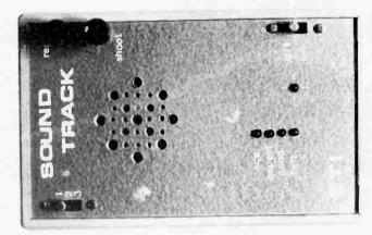
The on-off switch, SW2, is mounted on the front panel at the bottom righthand side such that it will be over R38, 41-43.
