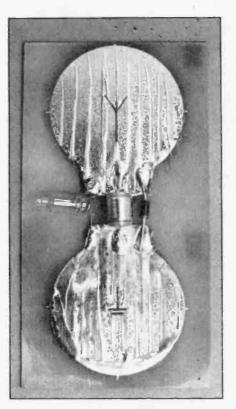
The assembled blinker, which we tinned with solder to avoid sweaty finger marks and oxidation. The cathode of D8 is at the bottom
