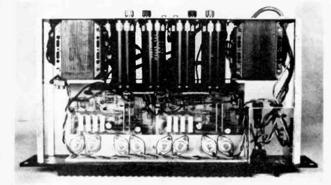
A general view showing the internal layout of the amplifier. Toroidal transformers can be used instead.
