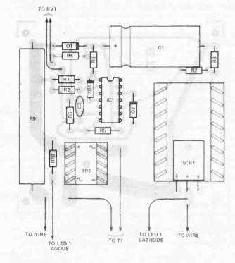
Fig. 2 Component overlay for the polystyrene cutter.
