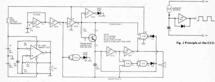
Fig. 1 Circuit diagram of the Component Tester.
