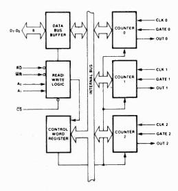
Figure 1. 8254 Block Diagram
