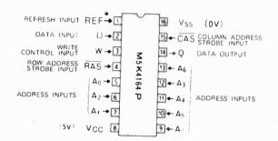
\* If the pin 1 (REF) function is not used, pin 1 may be left open (not connect).
