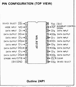
request flip-flop SR is set. Also, the strobed input STB is active, the data inputs  $DI_1 \sim DI_8$  are latched in the data latches, and the service request flip-flop SR is reset.
