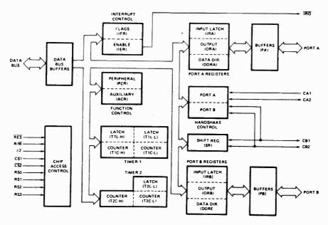
Figure 1. R6522 Block Diagram
