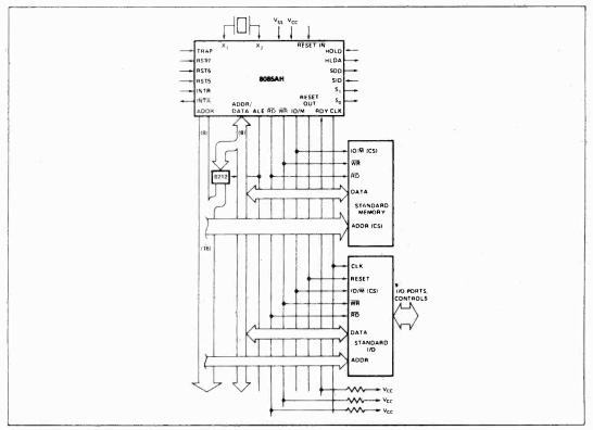
Figure 9. MCS-85® System (Using Standard Memories)
