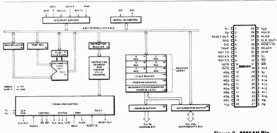
Figure 1. 8085AH CPU Functional Block Diagram
