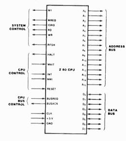
Figure 1. Pin Functions
