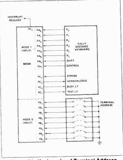
Figure 21. Keyboard and Terminal Address Interface
