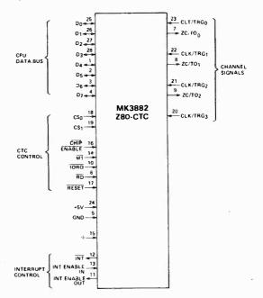
required to interface with a wide range of devices. In most applications, little or no external logic is required. The Z80-CTC utilizes N-channel silicon gate depletion load technology and is packaged in a 28-pin DIP. The Z80-CTC requires only a single 5 volt supply and a one-phase 5 volt clock.
