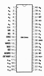
Transfers can be done between any two ports (source and destination), including memory-to-I/O, memory-tomemory, and I/O-to-I/O. Dual port addresses are automatically generated for each transaction and may be either fixed or incrementing/decrementing. In addition, bit-maskable byte searches can be performed either concurrently with transfers or as an operation in itself.
