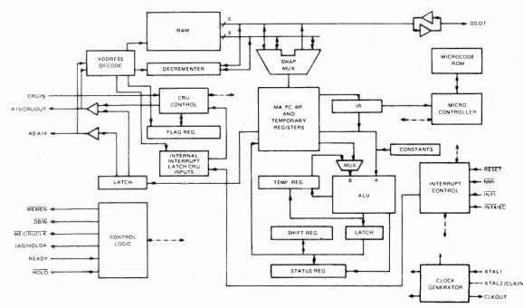
FIGURE 3 - TMS9995 BLOCK DIAGRAM
