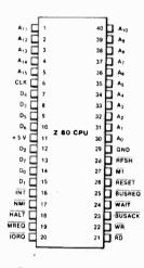
Figure 2. Pin Assignments
