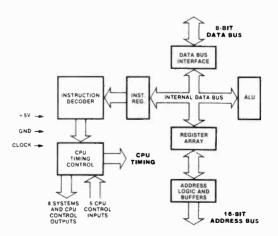
Figure 3. Z80 CPU Block Diagram
