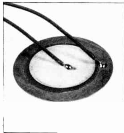
Soldering to the piezo transducers.
