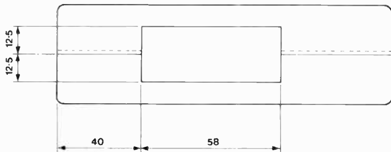
Figure 4. Battery box aperture. The cut-outs must be made in the top moulding end with the groove joint and bottom moulding end with the tongue.
