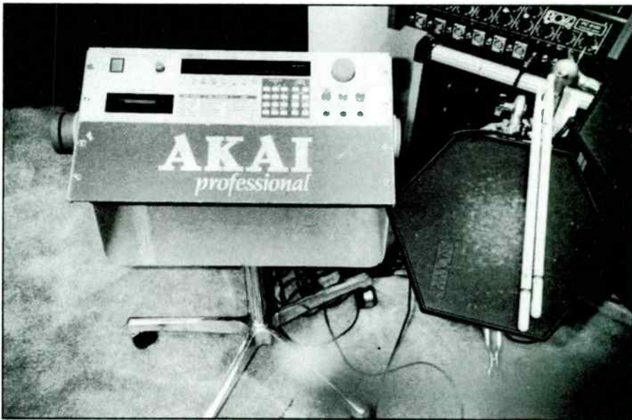
Updating drum tracks is now an important studio use for multi-timbral samplers like Akai's S900; latest trigger-in mods to this machine enable percussion parts to be tapped in 'live' from a suitable pad
