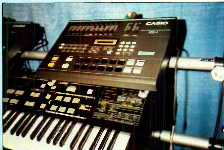
Casio RZ1 drum machine caused a stir at both Anaheim and Frankfurt, offers digital preset voices and user-sampling facilities at sensational RRP of under £400
