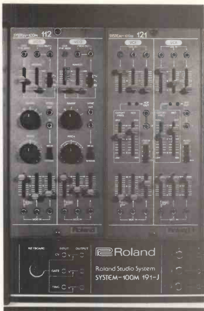
VCO and VCF modules.
