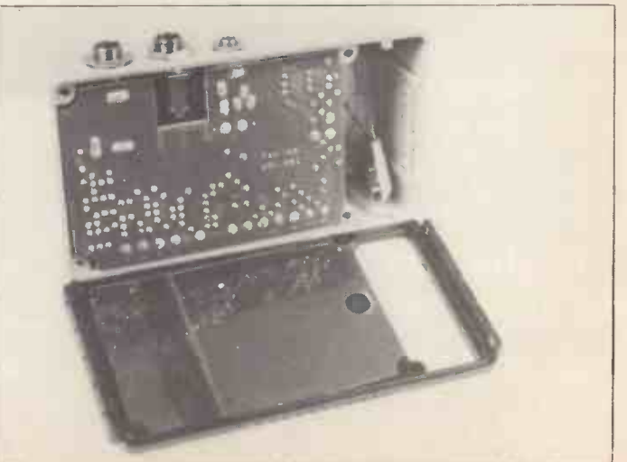
PCB fitted and insulation added to the bottom plate (Steps 17-18).
