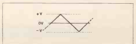
Figure 4b. Typical output from LFO.
