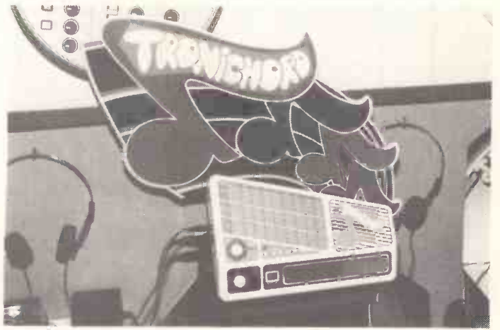
Suzuki's Tronichord, developed from the popular Omnichord. All controls are now touch sensors rather than a mixture of sensors and buttons, and 27 chords are available together with 'Sonic Strings' which can be played by hand or with a conductive plectrum. Suzuki, 443 Rydke-Cho, Hamamatsu, Japan.
