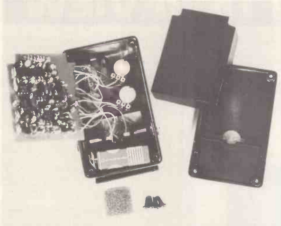
Internal construction of Loco effects.
