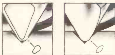
Shure's Hyperelliptical stylus design.
