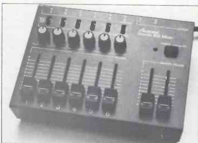
Steps 22-30. Sockets, mains cable and knobs added to complete the mixer.
