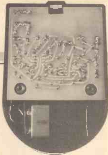
Internal view of the Soft Distortion Pedal, PCB in position.
