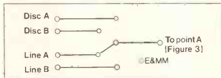
Figure 1. Monitor source selection by rotary switch.
