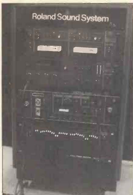
Roland Sound System Rack unit. Note the cartridge units.
