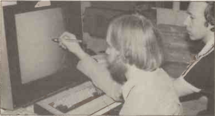
Using a light pen to inspect and modify circuits and IC layouts.
