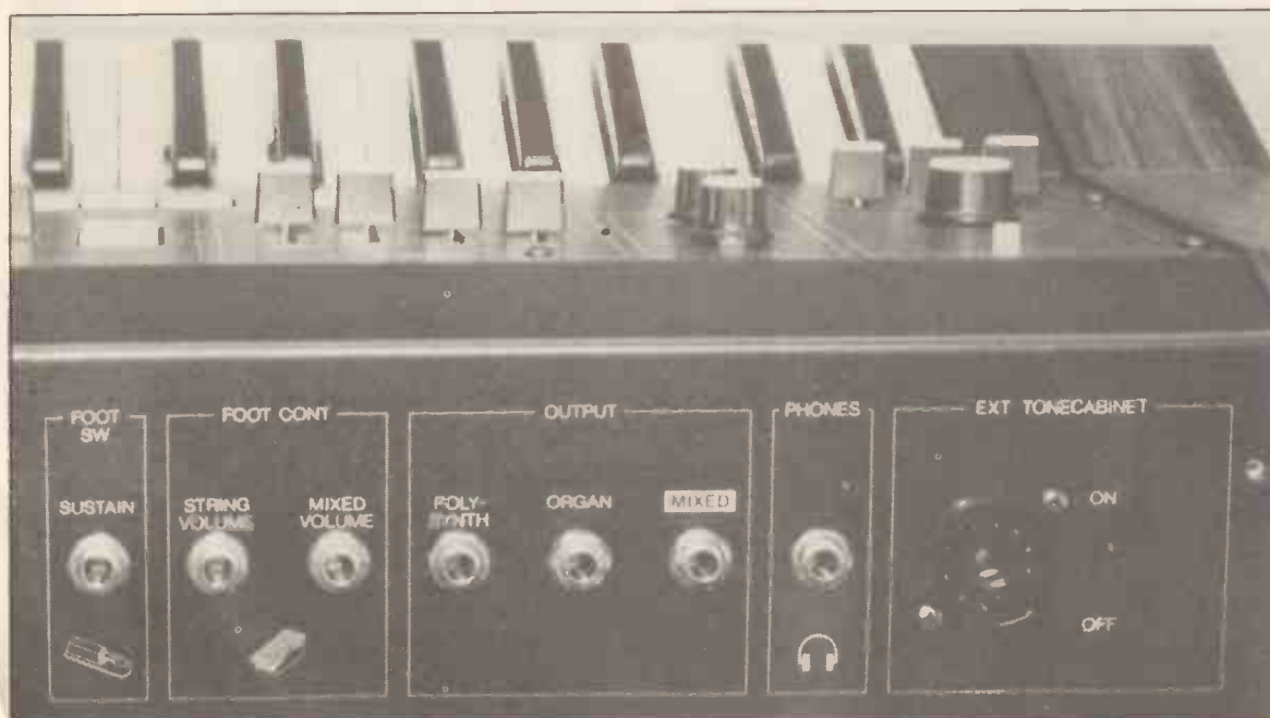
Fig. 6. Rear connection panel.
