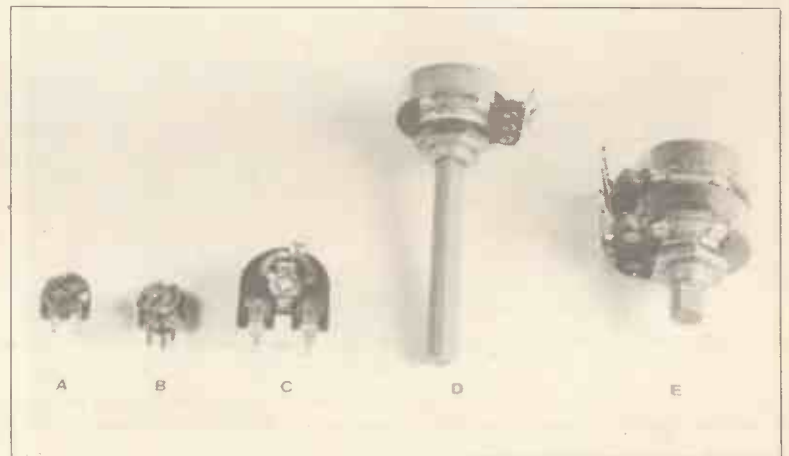
Examples of potentiometers: (a) 0.1W horizontal preset, (b) 0.1W vertical preset, (c) 0.25W horizontal preset, (d) carbon potentiometer, and (e) dual gang carbon potentiometer.
