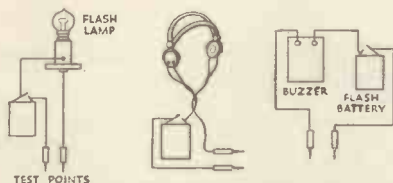
FIG. 1.—How a flash lamp, headphones and a buzzer can be used for circuit testing. Only a click is obtained in the headphones, but the lamp and buzzer give continuous indication.
