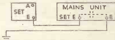
FIG. 17.—Essential safety condenser for the earth connection of a D.C. mains unit.
