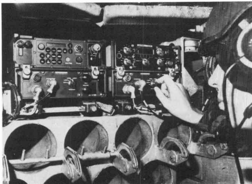
The Marconi SCIMITAR-H h.f. set (left) and the SCIMITAR-V v.h.f. set (right) are seen fitted inside a Chieftain Main Battle Tank.
