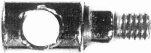
Fig. 2. Bicycle brake adjuster lug. (By courtesy of T. I. Raleigh Ltd, Nottingham.)
