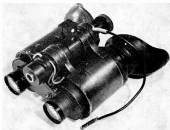
Fig. 14. A pair of goggles, containing two channel image intensifiers, suitable for head mounting.
