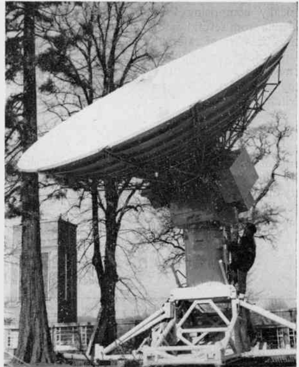
The first 21 ft (6.4 m) diameter dish for Skynet at a G.E.C.-A.E.I. (Electronics) establishment.
