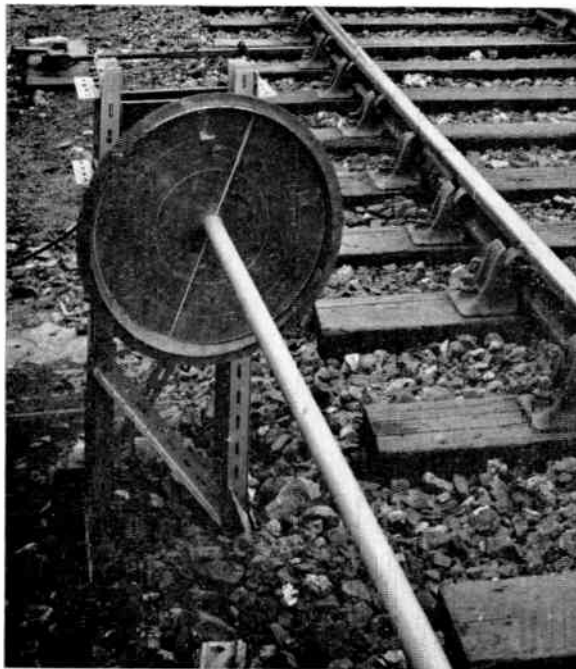
Fig. 1. Experimental trackside axial cylindrical surface waveguide designed by British Railways and Ferranti Ltd.
