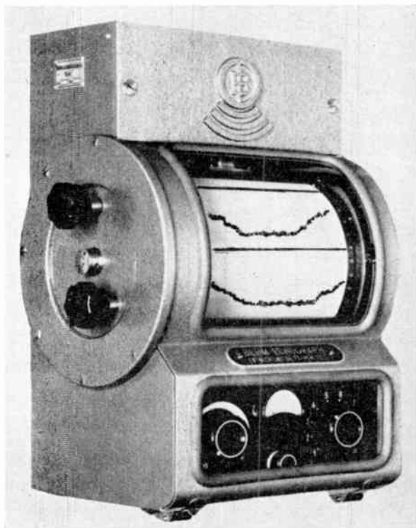
Fig. 10. Rotograph for recording transverse profiles in 0.2 seconds.
