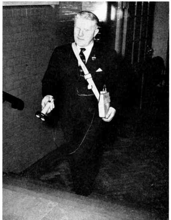
The blind guidance aid in use. The hand-held "torch" contains two piezo-electric transducers. A hearing-aid type earphone is used.
