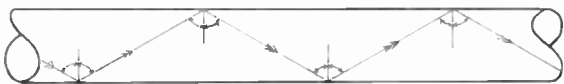
Fig. 1. Total internal reflection of a ray of light in an optical fibre.
