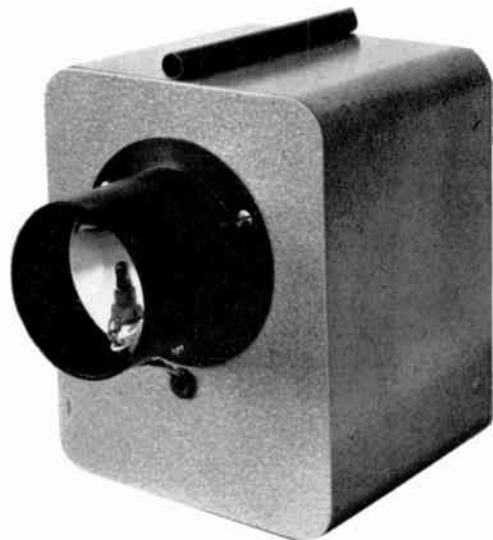
Fig. 1. A miniature photophone receiver using transistors and flash-lamp batteries.
