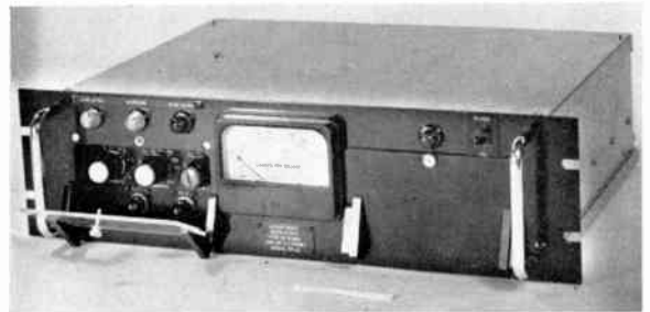
Fig. 2. Logarithmic ratemeter, A.E.R.E. type 1598A.
