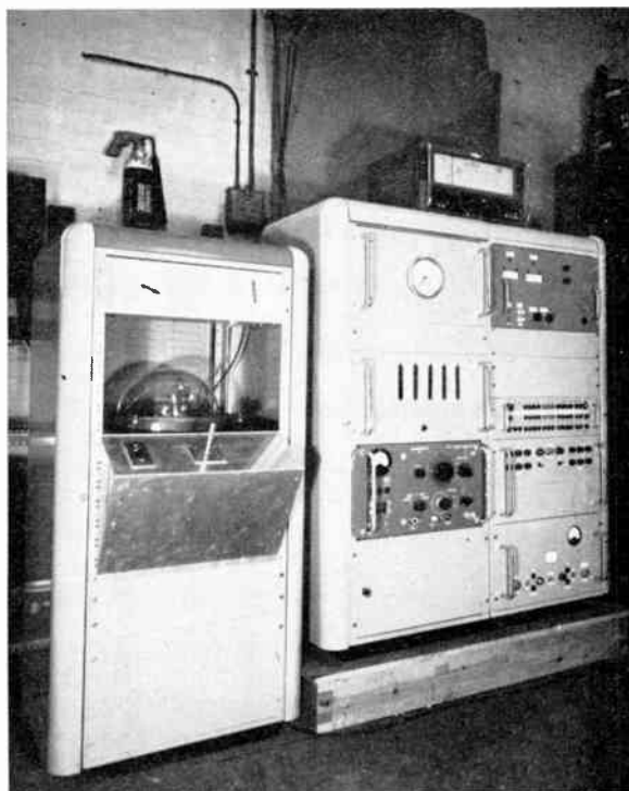
Fig. 6. Aerial control unit. The aeri- als shown in Fig. 5 may be pointed towards the satellite with the aid of this control unit.
