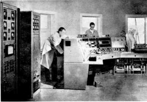
Fig. 7. Control desk of telescope on top floor of supporting tower.
