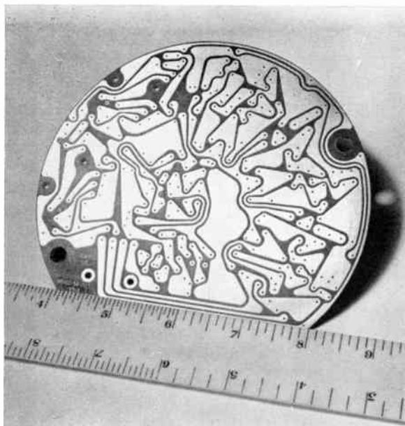
Fig. 2. A printed circuit card as used in the x-ray spectrometer.
