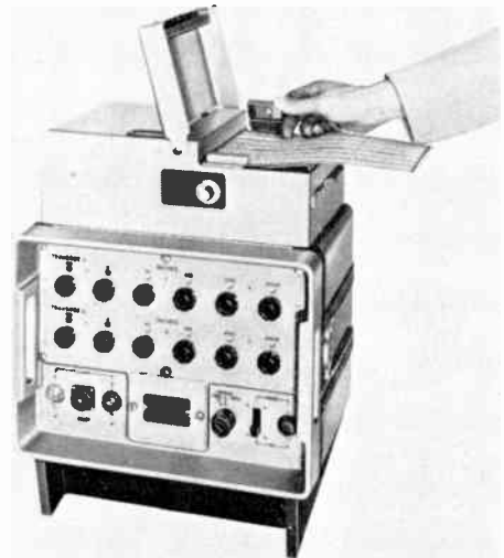
Fig. 2. Control unit and card reader of Ekco machine tool control equipment.
