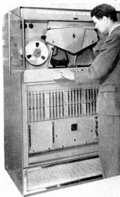
Fig. 20. Prototype tape unit with lower doors removed.
