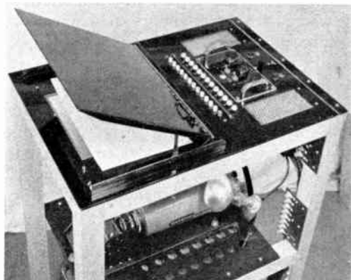
Fig. 2. A document viewing console, designed for transmission of bank statements, incorporating a vidicon camera. Camera controls and monitor selector switches are mounted in the top of the console.
