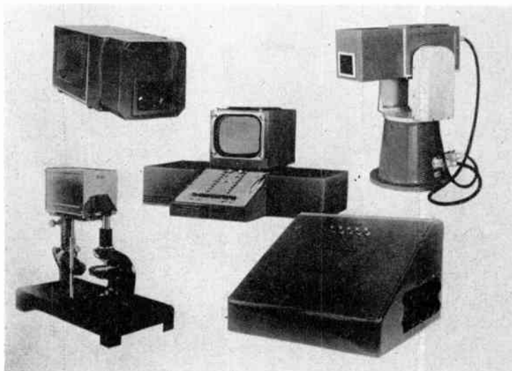
Fig. 3. Various appliances extending the application field of the IITY-0 and IITY-2 television sets (camera with optical head, camera with rotary gear, camera with microscope, switching consoles for 5 and 18 cameras).
