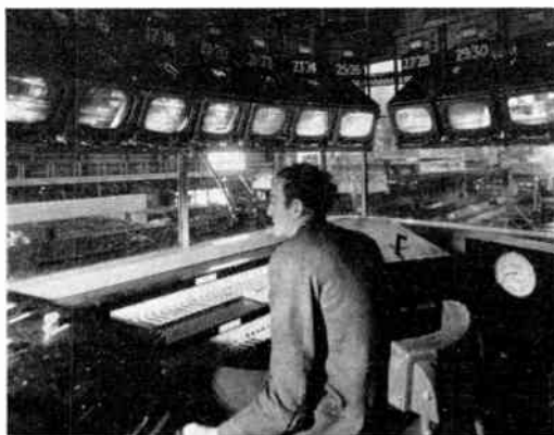
Fig. 3. Industrial television in use at the Steel Company of Wales for the remote control of the ingot buggy and shuttle car feeding ingots into the slabbing mill. Fifteen cameras and monitors provide a continuous view of approximately 700 feet of track.
