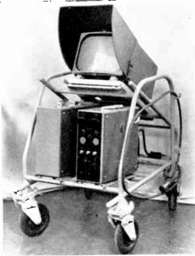
Fig. 5 The control and viewing equipment employed with a reactor camera.
