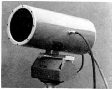
Fig. 2. General purpose industrial camera, contained in a sealed enclosure, and fitted with a remote controlled pan-and-tilt head.
