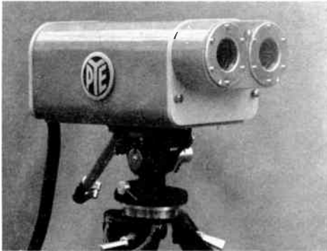
Fig. 3. A sealed stereoscopic camera for use in connection with master/slave manipulator.
