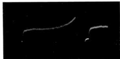
Fig. 20. Dark current—line direction. Slope of 45° represents \delta V/\delta H=0.2 .
