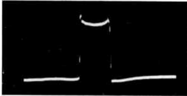
Fig. 13. Vertical resolution, edge effect and halo. Target/mesh potential 2.0 V. Below knee.
