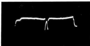
Fig. 6. Sensitivity and contrast law measurement. Electronic and camera pulse after superimposition, before complete cancellation.
