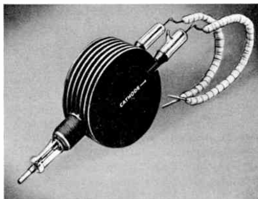
Fig. 2. An early production magnetron
