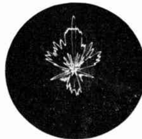
Fig. 18.—Combined horizontal interrogator and control patterns, illustrating the screening of the control pattern by the interrogator array when the control radiators are close together as shown in Fig. 17.
