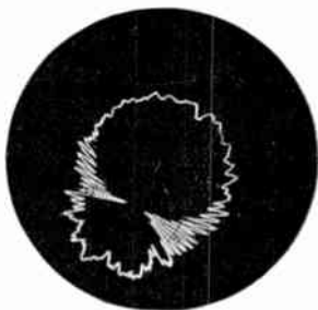
Fig. 20.—Pattern for forward and rear control radiators spaced apart and radiating coherently.
