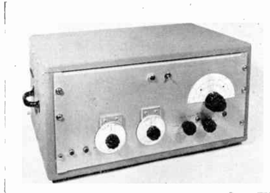
Fig. 12.—Photograph of the high-frequency apparatus. From the left to the right : terminals for the two output voltages, amplitude dial, phase dial, phase-interval switch, terminal for controlling symmetry of buffer stages, frequency range switch, terminal for controlling symmetry of 3-phase oscillator. Above frequency range switch : frequency dial.
