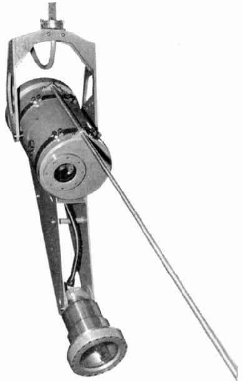
Fig. 7.—Deep sea unit with remotely focused lamp and combined lifting rope and supply cable.
