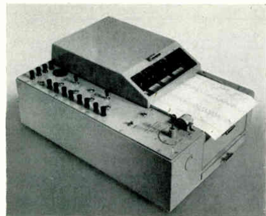
Fig. 8.—A four-channel direct-writing pen recorder in which the ink record is immediately available for study and measurement.
