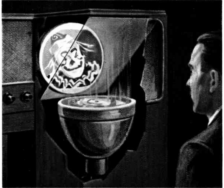
Plate B. The two-colour picture-reproducing system. Two kinescopes are used with the appropriate colour phosphors, and no filters are required.
