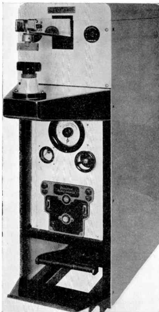
Fig. 4.—High-frequency jig or bar welder, 350 watts output, frequency 28 Mc/s.
