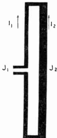
Fig. 2.—Folded dipole of two elements of unequal diameter.
