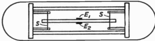
Fig. 4.—Luminous quartz resonator for wavemeter calibration.
