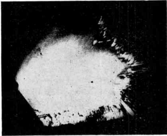
Fig. 2.—Quartz slab illuminated by polarized light viewed through a Nicol prism. The twinned portions lie close to three edges.
