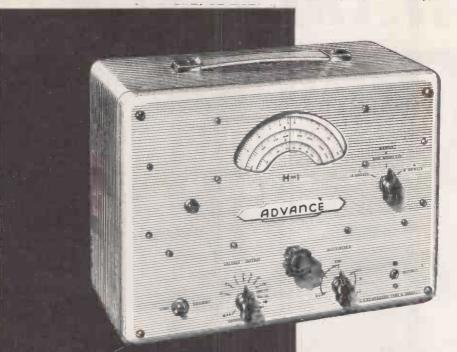
The Advance type H1 Audio Signal Generator completely covers the unusually wide range of 15 c/s to 50,000 c/s. It is characterised by its extremely low distortion and level output over the entire range ; provides both sine and square wave output. A robust, reliable and accurate instrument for the discriminating service engineer • Accuracy ± 1%, ± 1 c/s. • Distortion less than 1% at 1,000 c/s. • Output from 200 microvolts to 20 volts with accuracy of ± 2 db. • Weight 14 lb. • Size 13!\*×10!"×8"
