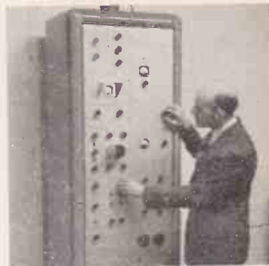
R. MacPherson, publicity and sales manager of Peto Scott, adjusts the flying-spot scanner which was used to provide still pictures for the TV sets on the Peto Scott stand.
