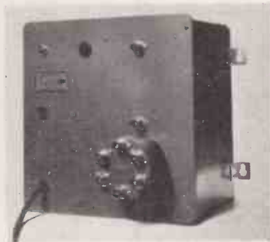
In addition to three Band III converters, Spencer-West exhibit this 12-outlet distribution unit for Band III.
