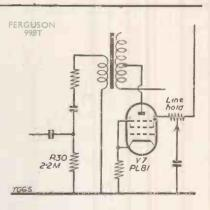
to about  $4M\Omega$ . In replacing this component it is advisable to use a resistor of solid carbon 1 watt type.—M.A.H., Exeter.
