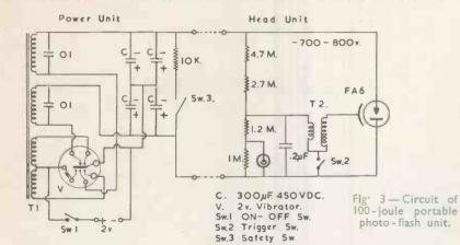
Almost all types of speedlight apparatus in this country are positively earthed. When tracing the faults in power supplies remember: The voltages employed are very high (often over 1,000 volts) and due to the high tank condenser could be lethal. Before attempting any repairs always discharge the tank condenser through a 5 or 10 watt resistor of value 1 to 5 kilohms, until the tank condenser is fully discharged.
