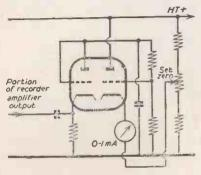
Fig. 5. A typical indicator for recording level.
