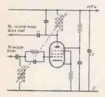
Fig. 4. A typical h.f. oscillator circuit.
