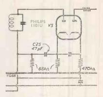
voltage tests showed no obvious discrepancies. After this, attention was directed to the sound detector stage and in checking over the components it was found that the 47pF filter capacitor C25 had developed a leak of around  $30k\Omega$ —R.R., Mansfield, Notts.
