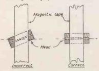
Fig. 2. Incorrect and correct alignment of the recording head.
