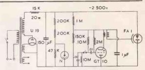
the common earth. If triggering circuit is in order, a spark should jump across when pressing switch.
