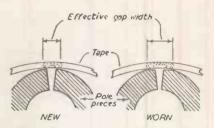
Fig. 3. Showing the increase in effective gap width due to wear on the pole pleces.
