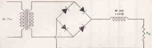
Fig. 4. Four of the new EW54 germanium junction rectifiers, when incorporated in a full wave bridge circuit operating into a resistive load with a smoothing choke, as shown, will provide an output of 20A at 50V.
