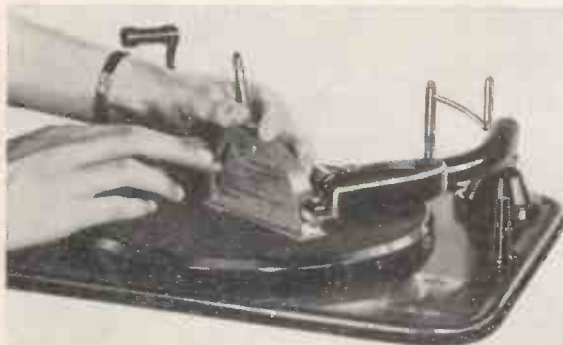
The Garrard stylus pressure gauge for microgroove pickups shown in use on a typical modern autochanger.
