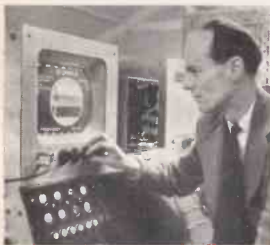
An engineer at the control desk of G9AED adjusting the uncorrected signal from the waveform generator. The picture as transmitted can be seen on the second monitor screen.
