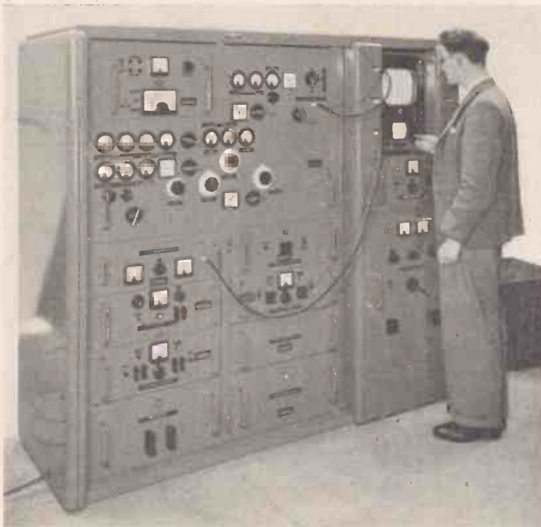
Outside television broadcasts from places not served by the special television cable will be considerably facilitated when this new transportable television transmitter, designed and produced by Marconi's Wireless Telegraph Co., Ltd., is brought into service by the B.B.C., as its small size and modest power requirements make it possible to install it in a single vehicle, which will carry also the fire-escape type extensible ladder for supporting the aerial. The new Marconi double-sideband transmitter is designed to radiate 350 watts within the frequency range 174 to 216 Mc/s.
